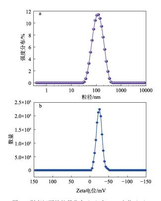
图 2 剥离蛭石的粒径分布(a)和 Zeta 电位(b) Fig. 2 Particle size distribution (a) and Zeta potential (b) of exfoliated vermiculite nanosheets
